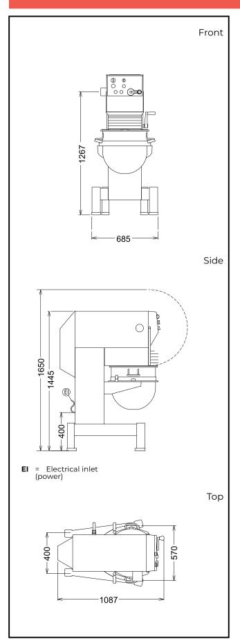
Electric 220-240/380-415 V/3 ph/50 Supply voltage: Electrical power, max: 1.54 kW **Total Watts:** 1.54 kW Capacity: ISO 9001; ISO 14001 kg/ Performance (up to): Cycle Capacity: 60 litres Key Information: External dimensions, 685 mm Width: External dimensions, Depth: 1087 mm External dimensions, **Height:** 1445 mm **Shipping weight:** 330 kg
